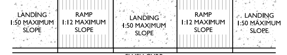
TRANSITION RAMP DETAIL NOT TO SCALE
