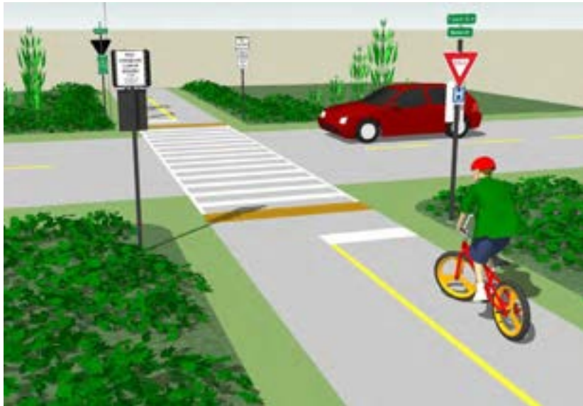
Fig. 9.10D. Trail Signs at Road Intersections Trail View
