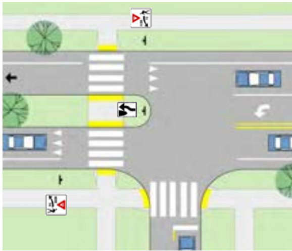
Figure 9.7A. Pedestrian Crossing Island
