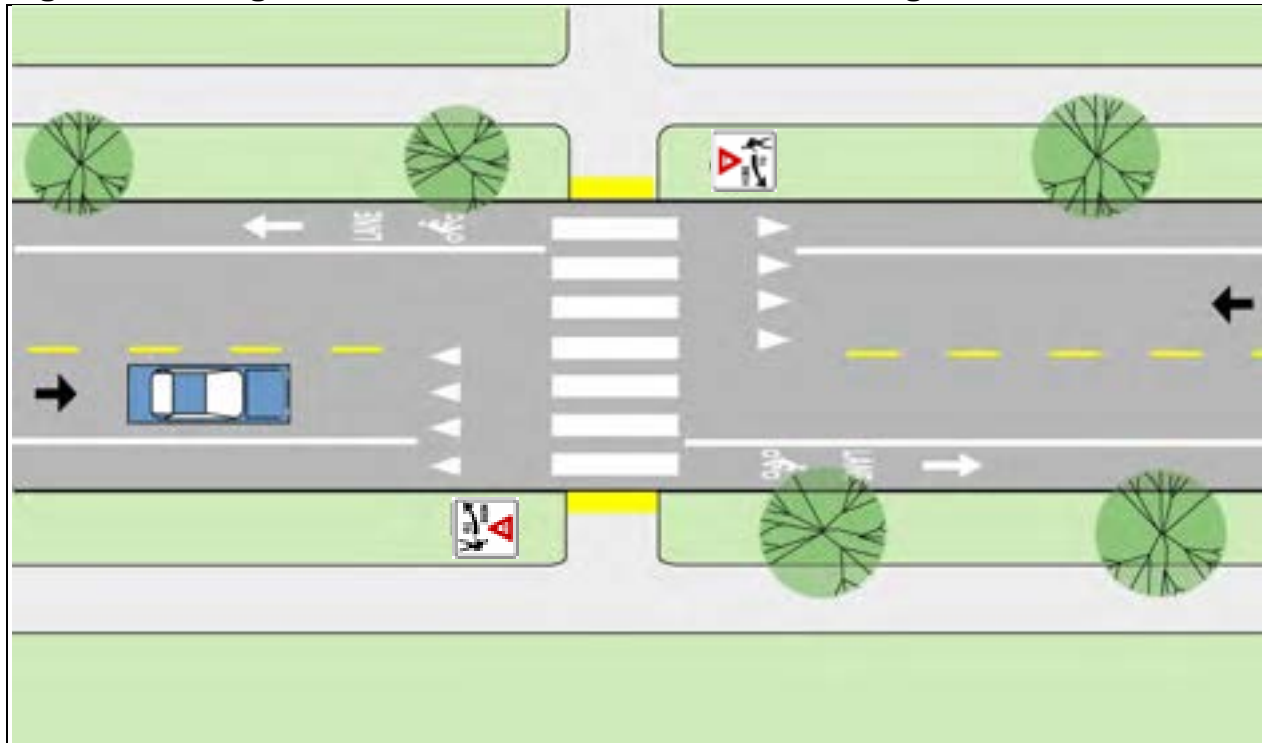
Fig. 9.7T. Unsignalized Basic Mid-block Crosswalk Design Guidelines
