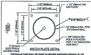
PARTICULAR CARE SHALL BE TAKEN TO PROVIDE SUFFICIENT PREHEAT OF THE THICKER ELEMENT FOR THE SOUNDNESS OF THE WELD. OTHERWISE, USE 5/16" (Imm) MIN. WEL
