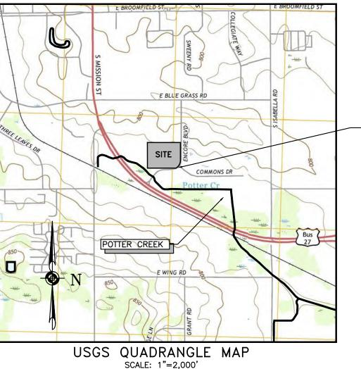
STORMWATER OUTFLOWS I & II STORMWATER FROM THE SITE DRAINS INTO A REGIONAL DETENTION SYSTEM LOCATED SOUTHEAST OF THE SITE. THIS SYSTEM DISCHARGES INTO POTTER CREEK, THE ULTIMATE RECEIVING WATERS. POTTER CREEK IS LOCATED APPROXIMATELY 650 FEET SOUTH OF THE SITE.
